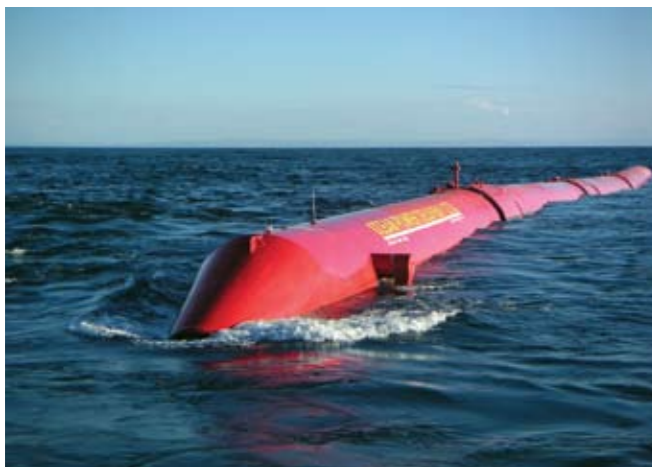
Pelamis 2-1 wave energy converter Source: The Crown Estate
