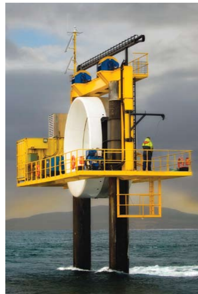
Open Hydro's Turbine test rig near Orkney off the coast of Scotland Source: The Crown Estate
