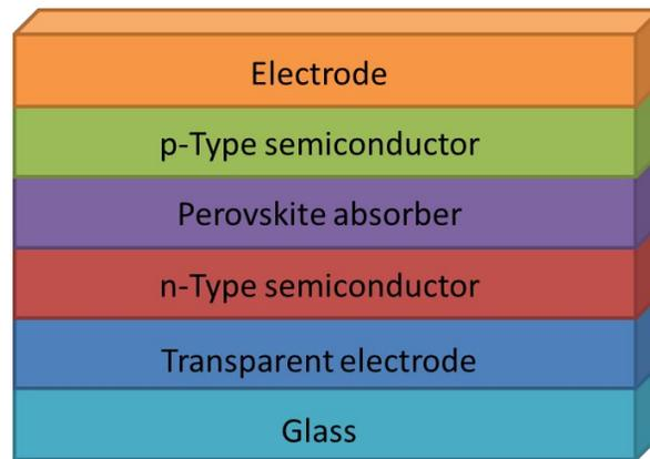
Figure 2: Perovskite solar cell structure
