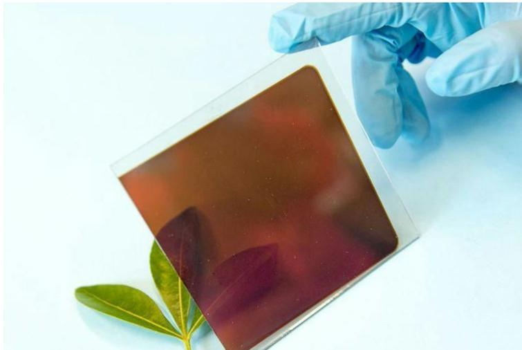
Figure 1: A perovskite solar cell prototype [2]
