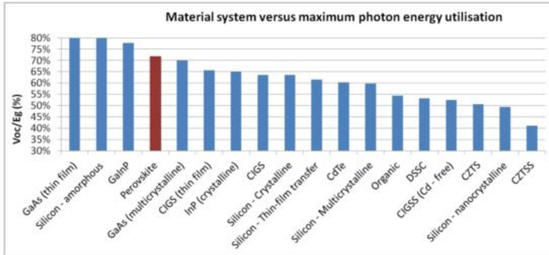
Figure 4: Maximum photon energy utilization for various solar cell technologies [6]
